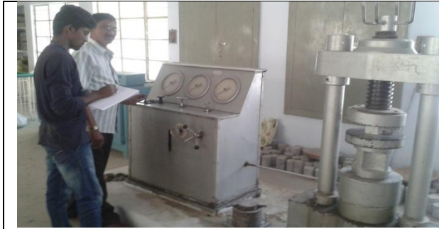
Figure-3: Testing of mortar cubes.
