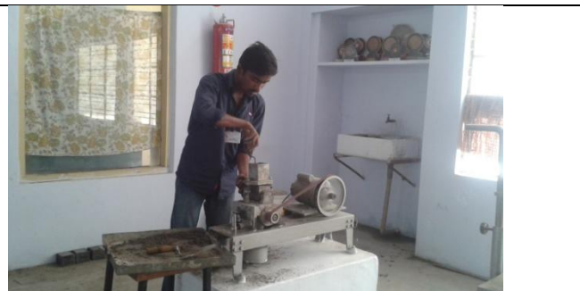
Figure-2: Casting of mortar cubes.
